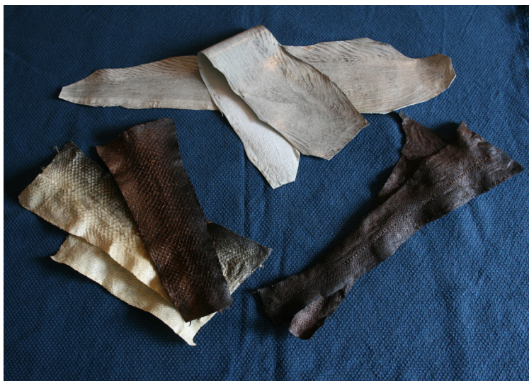
Figure 2: Examples of finished fish leather. Commercially available catfish leather (top), two oil tanned and one vegetable tanned salmon skins (bottom left) and two vegetable tanned rainbow trout skins (bottom right). © Roman Vávra.
