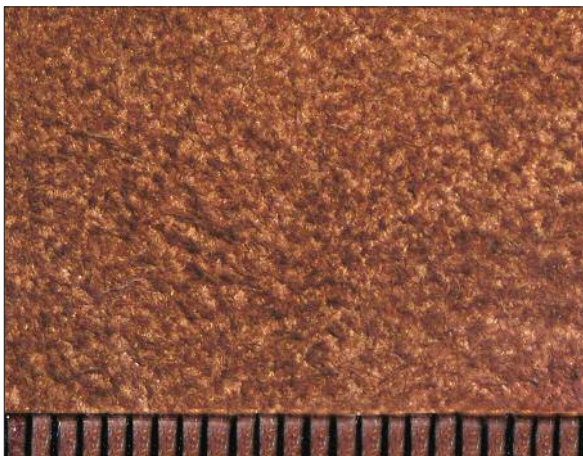
Fig. 4.22. The scraping quality of the flesh side of a tanned depilated skin from the Sámi culture defined as smooth and furthermore defined as even in colouring.
