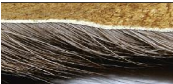
Fig. 4.16. Surface tanned/coloured leg skin (LS) of reindeer, reference sample LS-N13-01. Notice the low penetration of the vegetable tannin (willow bark extract). The thickness of the skin is 0.9-1.0 mm.
