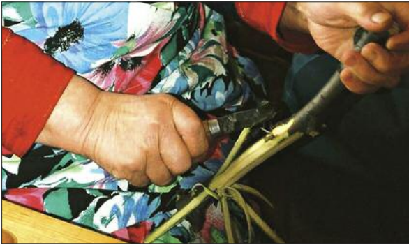
Fig. 3.31. Ellen Sara M. Sara, removing bark from a willow twig, using a bent knife as a debarking tool. Suotnju, Norway. March 2004.
