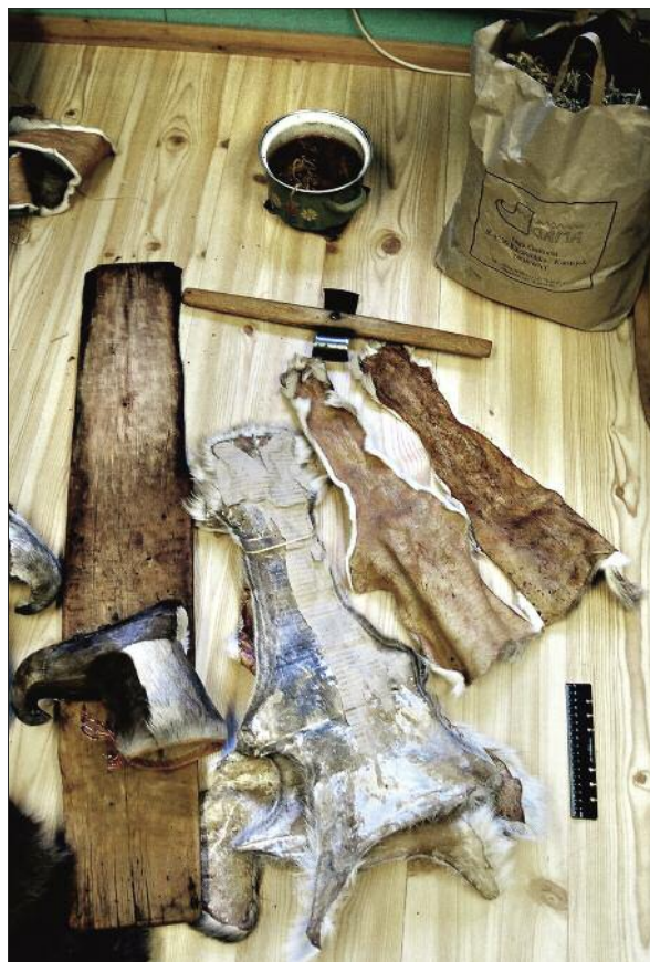
Fig. 3.34. Collection of tools and materials for the process of making short winter boots. From left to right: Scraping board, with a short boot lying on its side. Next to this, dried leg skins with remnants of paper attached to the flesh side and tanned leg skins. Above these leg skins there is a scraper with s-shaped blade. In the right upper corner a paper bag filled with willow bark scrapings and in the cooking pot next to it, boiled willow bark in water, ready to be used. In the house of Inga Guttorm, Karasjok, Norway, 2004.
