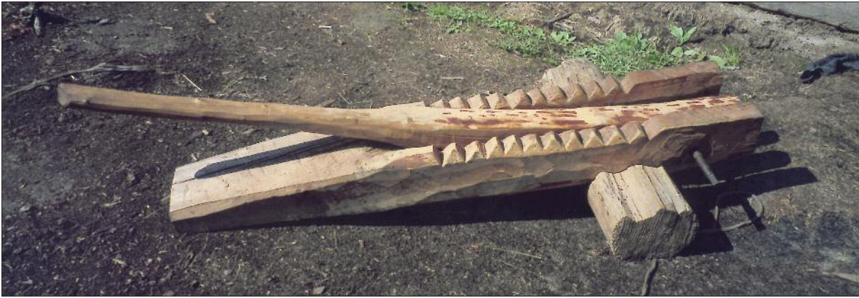
Fig. 3.49. A newly built skin press (talki), used to soften larger skins. Nichatka, Chita County, Russia, 2000.
